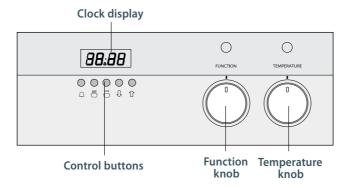
Figure 23 Main oven controls
